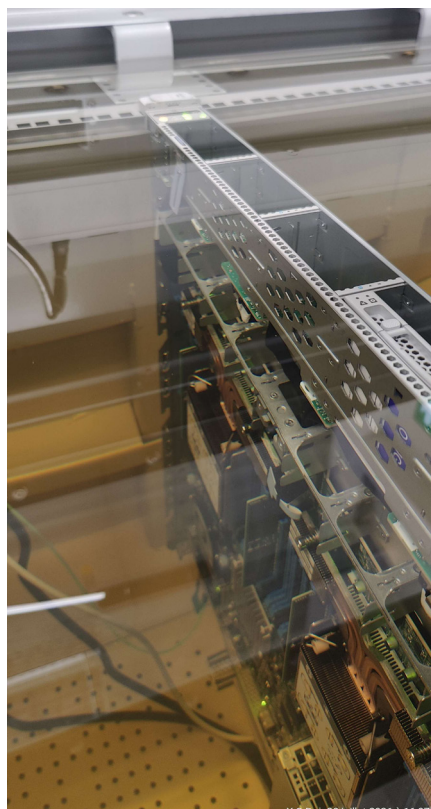
Cisco server in full immersion
